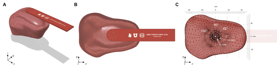
Figure 1. (A) Three-dimensional view of the tongue finite element model (FEM) with the user tongue depressor. (B) Top view. (C) Top view detail of the FEM dimensions length and width, angular arrangement of the surface electrodes and model mesh.
