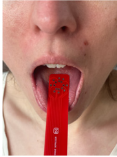
Fig. 8. Use example of the UTES and UTA for measuring tongue electrical properties (TEP) in a healthy subject. The UTA depressor was sterilized by autoclave.
