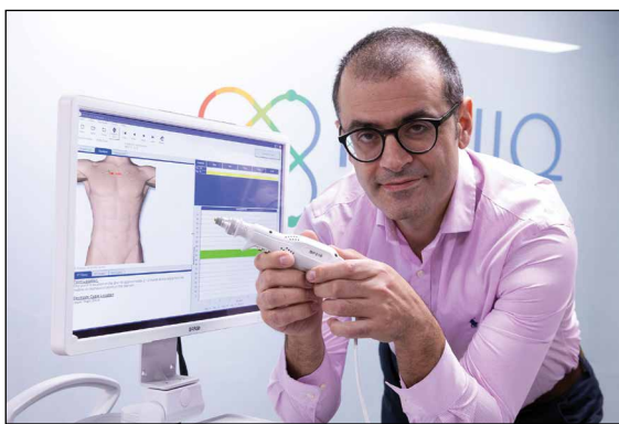
Figure 6. Benjamin Sanchez-Terrones, Ph.D., assistant professor of electrical and computer engineering at the University of Utah, is developing a noninvasive, radiation-free technology that detects changes skin resistance to electrical current flow to help detect breast cancer. It could have benefit for women who are too young to receive standard mammography screening, and for those who have dense breast tissue and receive inconclusive results from mammograms. (Photo courtesy of Dan Hixson/ University of Utah College of Engineering.)
